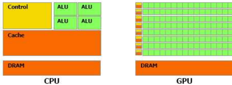
Figure 2.1: CPU versus GPU Chip area [21]
